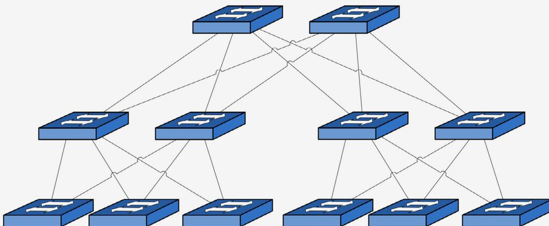
Figure 11 – Modified three-tier topology mask
